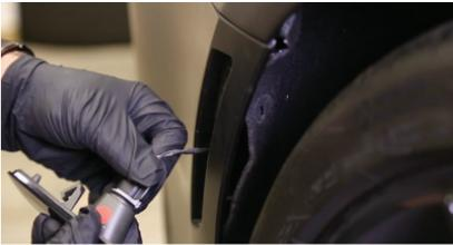
5. Twist the factory plug back into the new sidemarker to seal.
