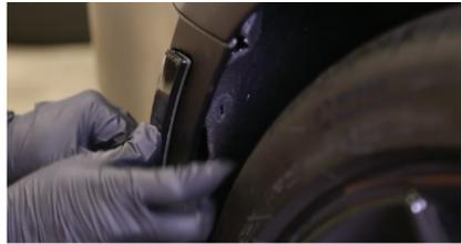
6. Place the sidemarker back into the bumper, clipping it into place. Reinstall the fastener. Repeat for all four sidemarker locations.
