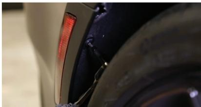
1. Using a T15 Torx Bit, remove the fastener located in the fender liner inside the wheel well. Pull back on the fender liner to access to the sidemarker.
