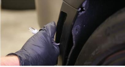
3. Twist the factory plug counterclockwise to remove from the sidemarker, and remove the bulb.
