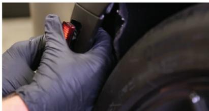
2. Remove the sidemarker by depressing the clip on the bottom side of the sidemarker, then pushing it out. Then depress the clip on the top side of the sidemarker to release it.
