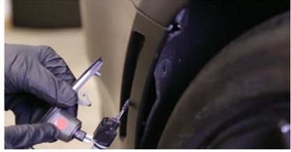
4. Plug the connector from your new sidemarker into the socket. Ensure you have the correct polarity by hitting the unlock button. If the sidemarker doesn't illuminate, flip the connector 180°.
